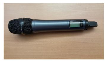
2 - To replace the batteries, unscrew the hand-held mic at the center, and insert 2 new AA batteries.
