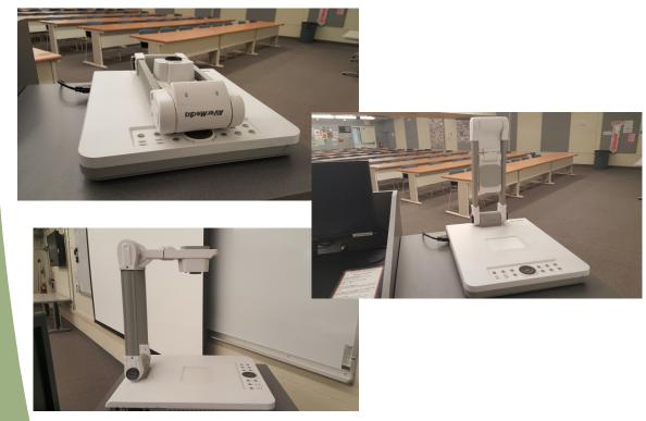
1 - Open the Aver Media camera (**top**) by pulling up on the top portion to full vertical height (**middle**). Then extend the lens horizontally (**bottom**).
