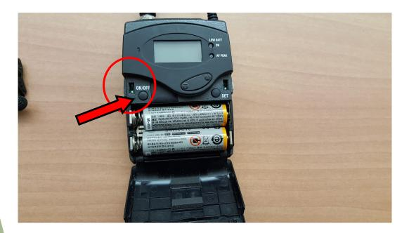
5 - This compartment allows access to change the batteries (two AA) when needed.
