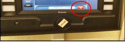
Press the red '**System Off**' button near the bottom right of the Control Box screen.
