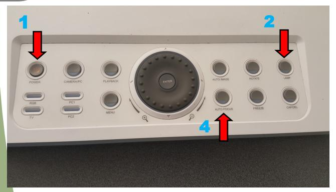
1 - Turn the camera on by pressing the '**Power**' button in the upper left corner.
