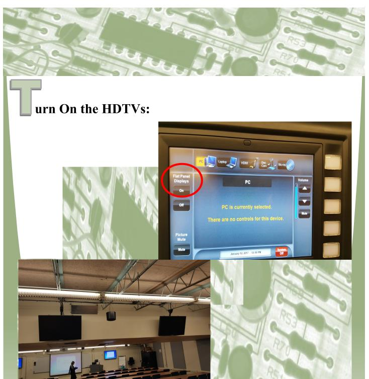
Once the main menu on the Control Box has loaded, you will find a button on the left hand side that says 'Flat Panel **Displays'**. Press '**On**' to turn on all of the TVs in the room (including the ones in the back of the room).
