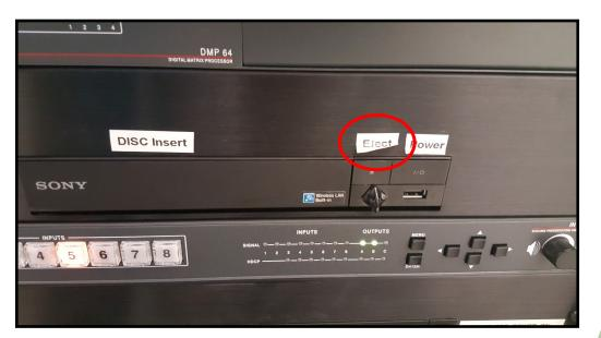
2 - Press the 'Eject' button on the Blu-Ray player to open the drawer. Insert the disk.Press the 'Eject' button again, or push the drawer in to close.
