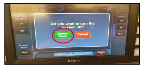
On the screen that comes up next, press the green '**Power Down**' button, which will automatically shut down all components. Please double check that the Document Camera is also off.
