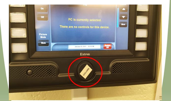
The round knob on the bottom, in the middle of the control box, adjusts the **VOLUME**.
